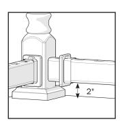
Measure between Posts subtracting 1/4" from total length, and if necessary cut Rails and Rail Insert to proper length by cutting an equal amount from each end. Do not cut through Baluster holes.
