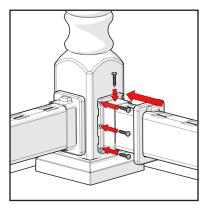
Tip: Cut a block to 2" and set Bottom Rail on it for support during installation
