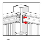
Place Top Rail with Rail Insert 36" or 42" (measured from the deck surface to the top face of the Rail), and onto Balusters. Fasten to center of Post with provided screws. Secure Bracket to railing then slide Screw Covers into place.
